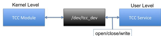
Figure 1: Module-Service Design
